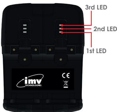
A fully discharged battery should be fully charged within 5.5 hours. While in a good condition, the battery run time will be 4 hours (assuming 50% idle time between scans).
