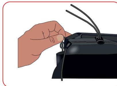
Now go round and check that all the side panels of the sun hood are wrapped over the sides of the scanner. Adjust the sun hood position so that the scanner buttons can be pressed through the transparent window panel.
